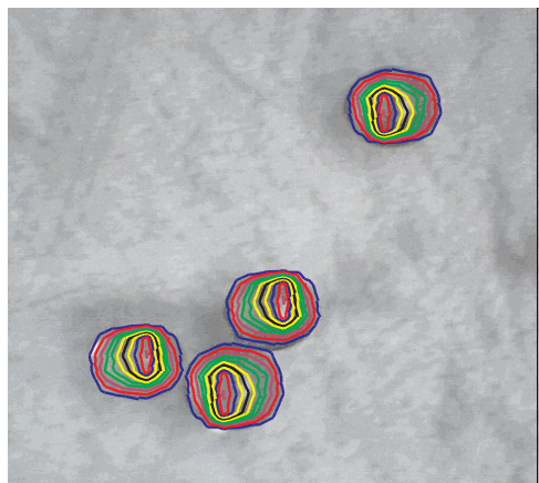
Figure 1. UV/Vis video image and IR reconstruction of four polystyrene resin beads with a diameter of about 80 \mu\text{m} . The IR map was obtained with a motor-driven x - y stage in combination with an IR microscope. For the reconstruction of the resin beads the integral of the polystyrene combination vibration at 1942\text{ cm}^{-1} was used.
